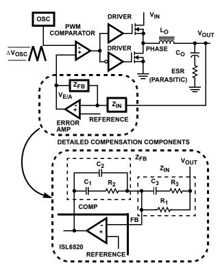
FIGURE 5. VOLTAGE-MODE BUCK CONVERTER COMPENSATION DESIGN
