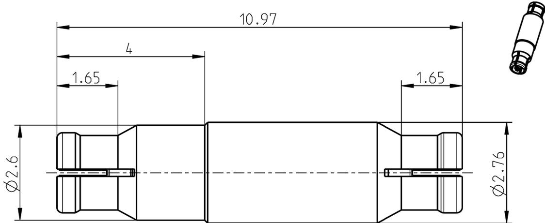
All dimensions are in mm; tolerances acc. ISO 2768 m-H
