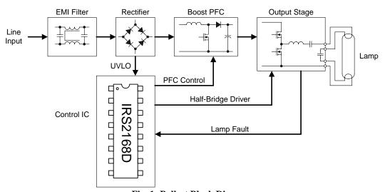
Fig. 1: Ballast Block Diagram
