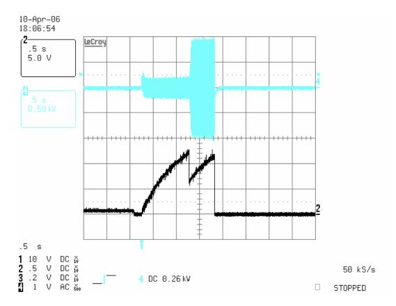
Fig. 10: CPH Pin Voltage (Black) and Lamp Voltage (Blue) During Lamp Non-Strike Fault Condition
