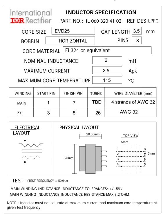
Fig. 5: Power Factor Inductor Specification
