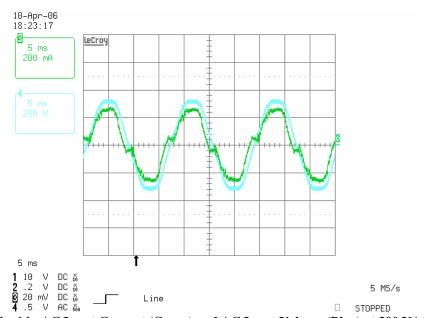
Fig. 14: AC Input Current (Green) and AC Input Voltage (Blue) at 290 VAC
