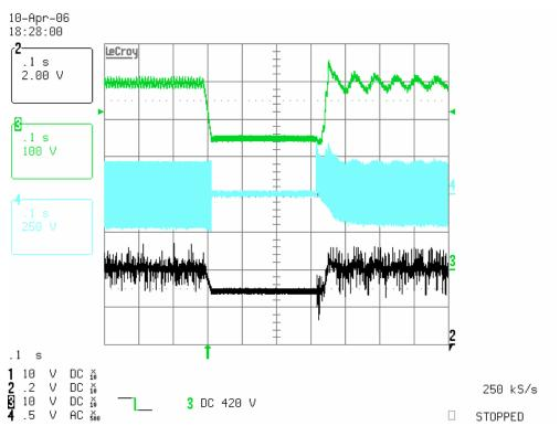
Fig. 16: VBUS Pin (Black), Lamp Voltage (Blue) and DC Bus Voltage (Green) During Momentary Interruption of the Mains
