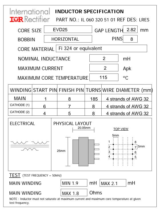
Fig. 6: Resonant Inductor Specification
