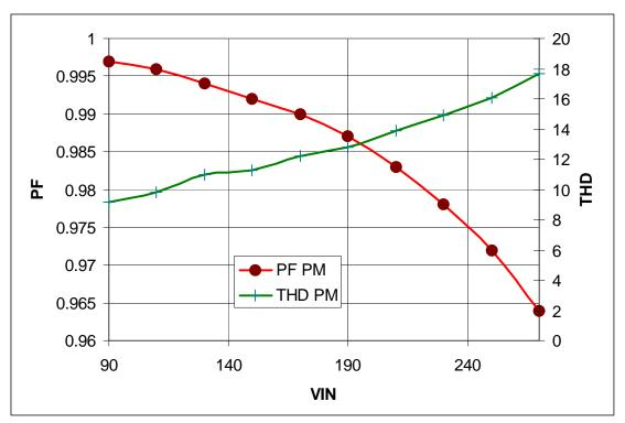
Fig. 2: PFC and THD Performances versus Input Voltage
