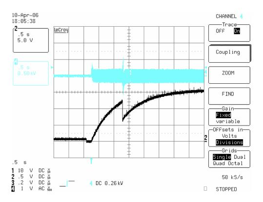
Fig. 7: CPH Pin Voltage (Black) and Lamp Voltage (Blue) During Normal Preheat, Ignition and Run Modes
