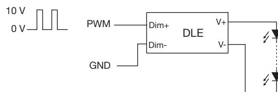
The dimmed output current is given by:
