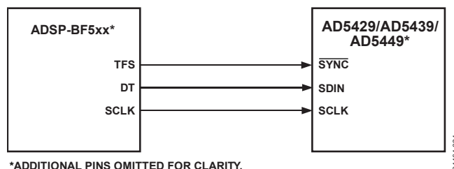
Figure 51. ADSP-BF5xx SPORT-to-AD5429/AD5439/AD5449 Interface
