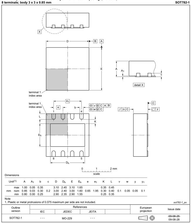
HVSON8: plastic thermal enhanced very thin small outline package; no leads; 8 terminals; body 3 x 3 x 0.85 mm
