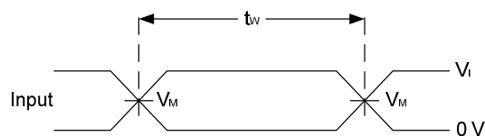
Voltage Waveform Pulse Duration
