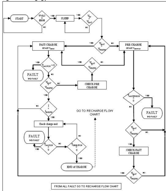
Figure 9. Charging process flow chart
