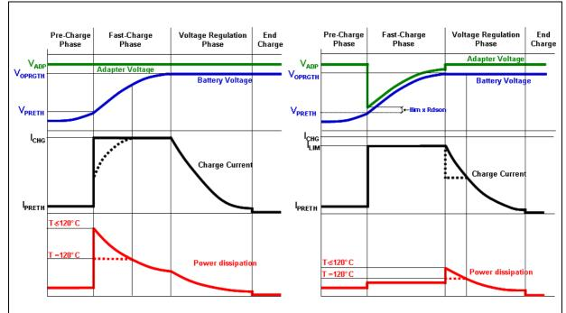
Figure 16. Power dissipation in both linear and quasi pulse modes with thermal loop
