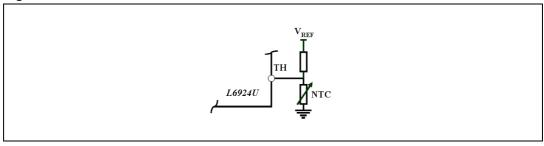
When the TH pin voltage rises and exceeds the  $V_{MINTH}$  = 50 % of  $V_{REF}$  (900 mV typ), the L6924U stops the charge, and indicates a fault by the status pins. The device re-starts to
