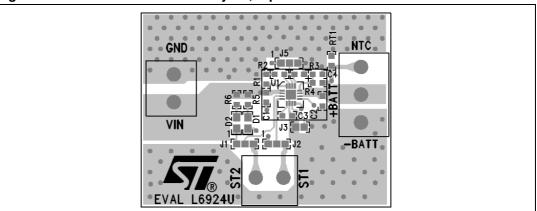
Figure 24. Demonstration board layout, bottom side
