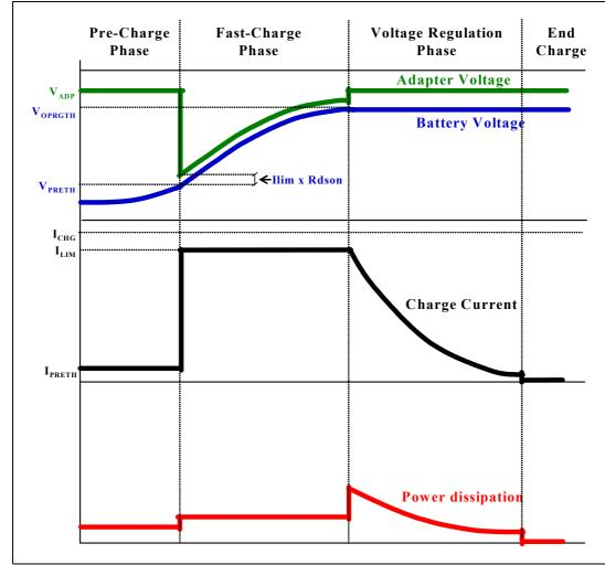
Figure 7. Typical charge curves in quasi pulse mode
