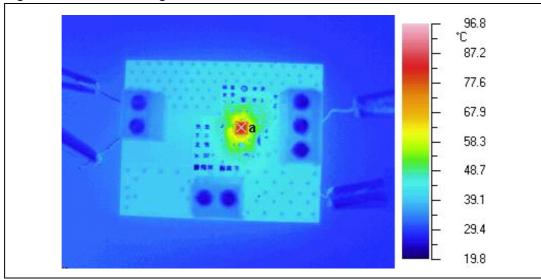
Figure 22. Thermal image of the demonstration board
