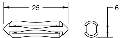
Consisting of a heat resistant body, the fuse element stretches over the exterior of the body from end to end. The body varies in color indicating the current ratings.
