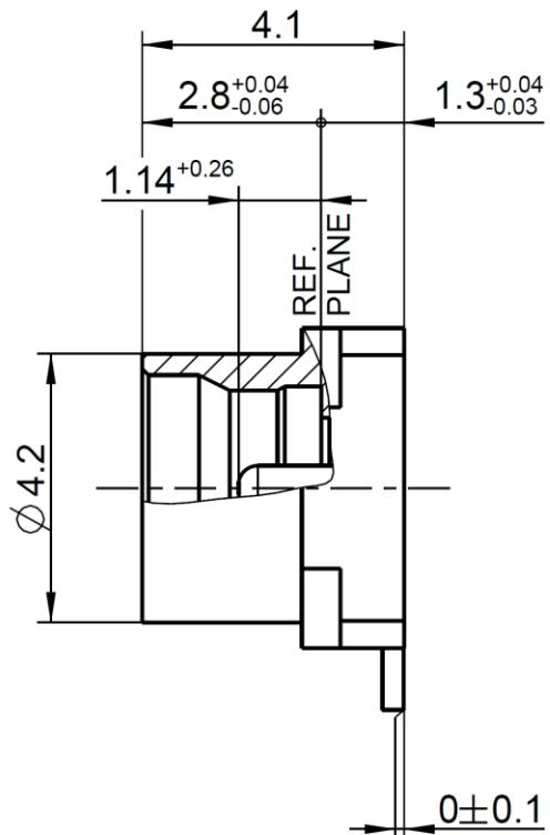
All dimensions are in mm; tolerances acc. ISO 2768 m-H
