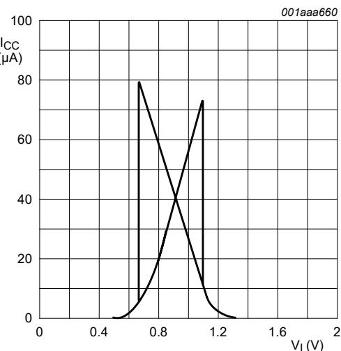
Fig. 11. Typical 74LV132-Q100 transfer characteristics
