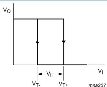
Fig. 8. Transfer characteristic
