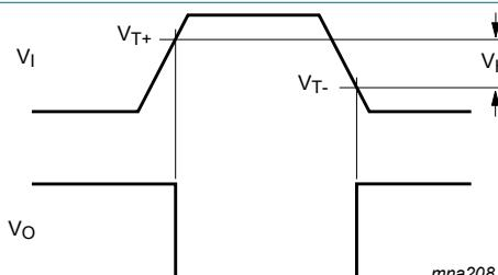
Fig. 9. Definition of VT<sub>+</sub>, VT<sub>-</sub> and VH
