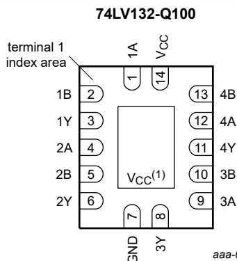
Fig. 5. Pin configuration SOT762-1 (DHVQFN14)
