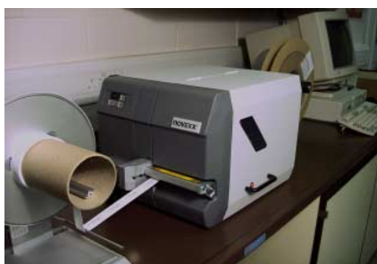
TMS 2000Plus in-line thermal transfer printer
