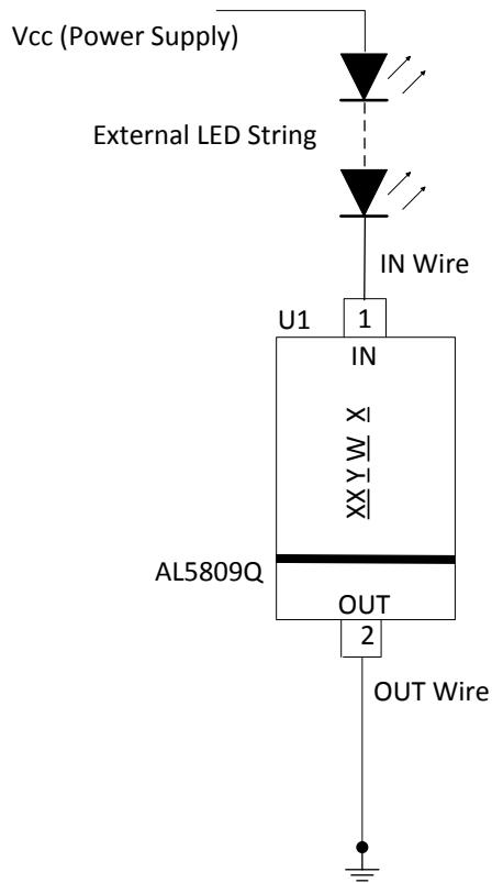
1. Depends on the current options, the evaluation board is as low side current LED configuration.
