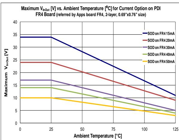
Figure 15. Maximum V<sub>InOut</sub> vs. Temperature
