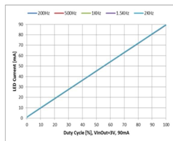
Figure 16 PWM Dimming 90mA vs. Duty Cycle
