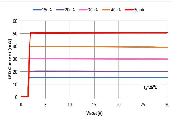
Figure 1. LED Current vs. V<sub>InOut</sub>
