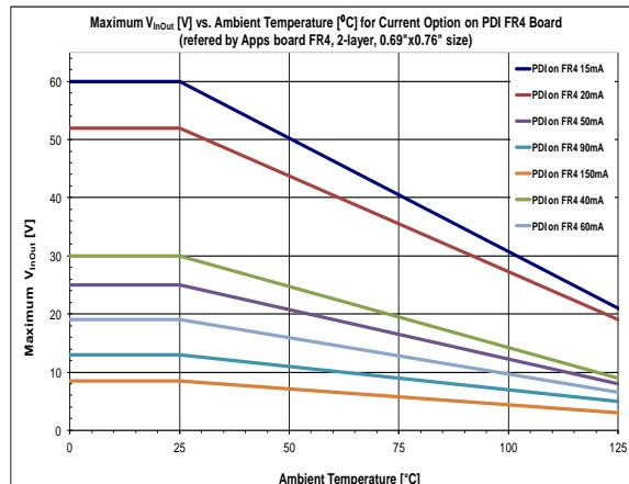
Figure 14. Maximum V<sub>InOut</sub> vs. Temperature
