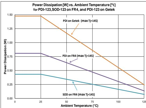
Figure 13. Power Dissipation vs. Ambient Temperature @  $T_J = 160^{\circ}\text{C}$
