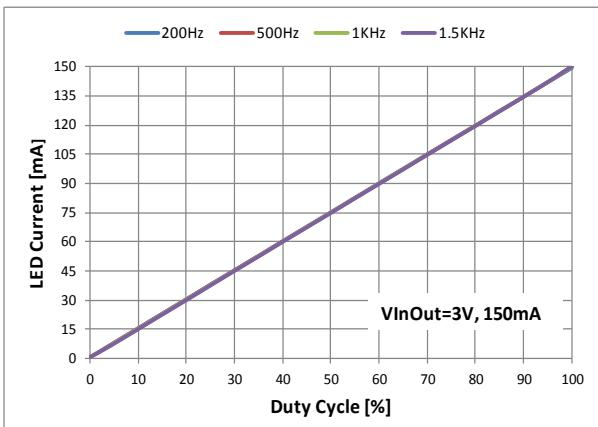
Figure 17. PWM Dimming 150mA vs. Duty Cycle
