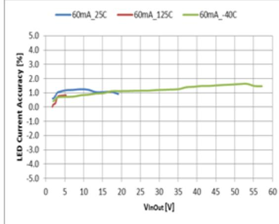
Figure 10 LED Current Accuracy (%) vs. VInOut across Temp
