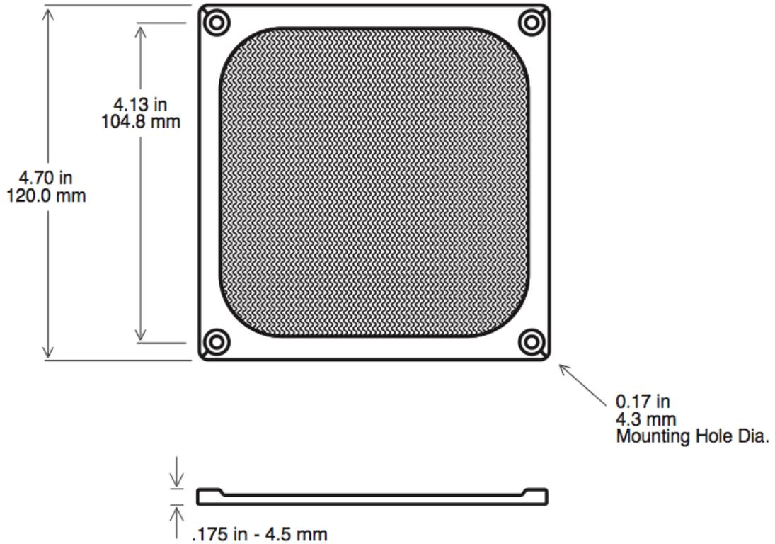
Aluminum/Stainless filters offer high levels of air passage while efficiently filtering contaminants and shielding EMI/RFI.
