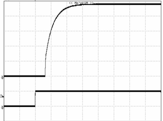
Figure 5: Turn-on transient at zero load current (20 ms/div). Top Trace: Vout; 10V/div; Bottom Trace: ON/OFF input: 5V/div.
