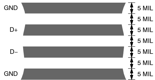
Figure 22. Typical Arrangement of Signal Tracks
