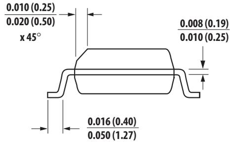
DIMENSIONS: INCHES (MILLIMETERS)  $\frac{\text{MIN}}{\text{MAX}}$
