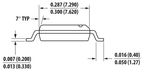
DIMENSIONS: INCHES (MILLIMETERS)  $\frac{\text{MIN}}{\text{MAX}}$
