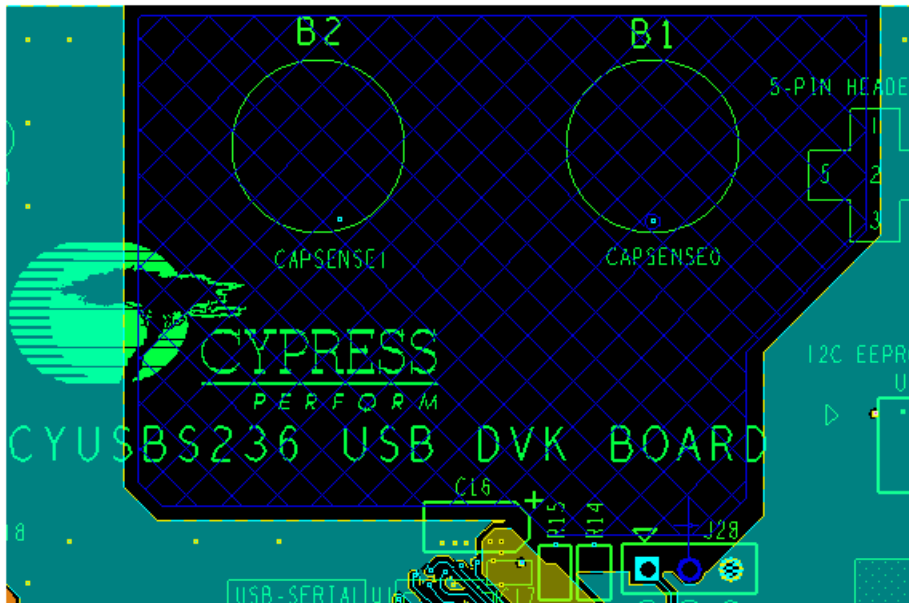
Figure A-11. CapSense Layout - Bottom Layer
