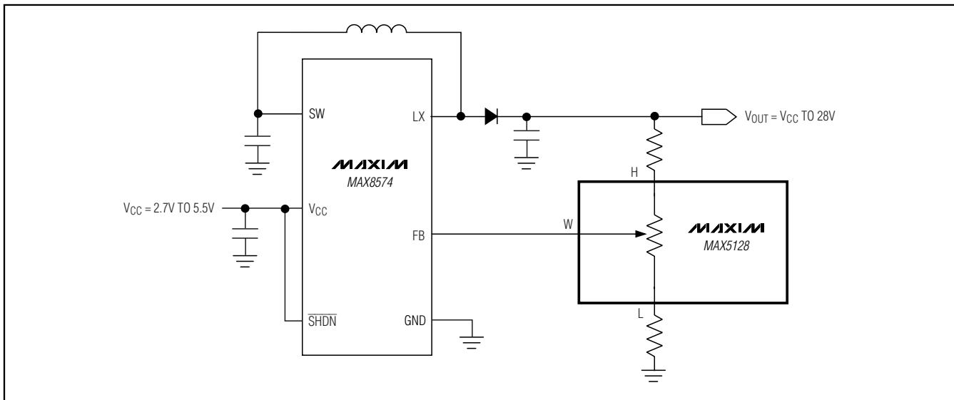
Figure 7. DC-DC Converter Using a Floating Potentiometer
