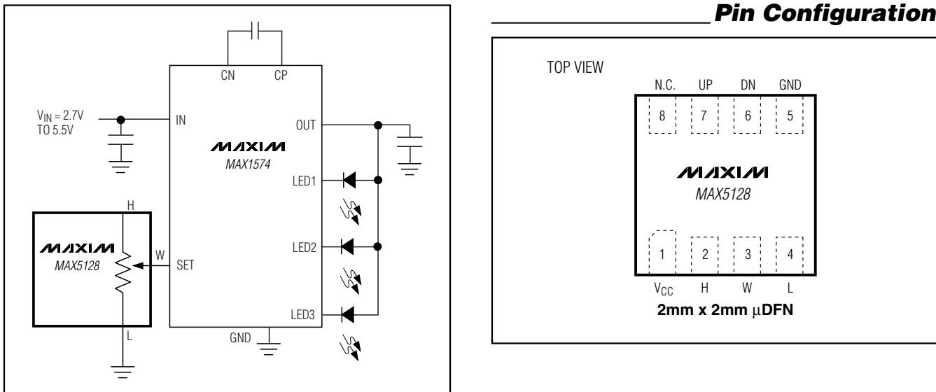
Figure 8. LED Bias Adjustment Using the MAX5128
