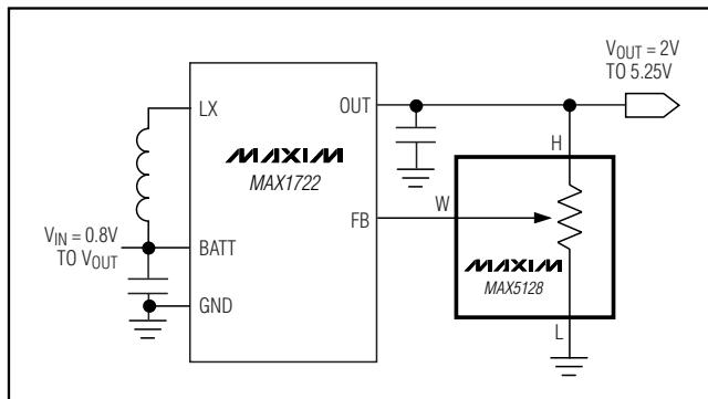
Figure 6. DC-DC Converter Using a Grounded Potentiometer
