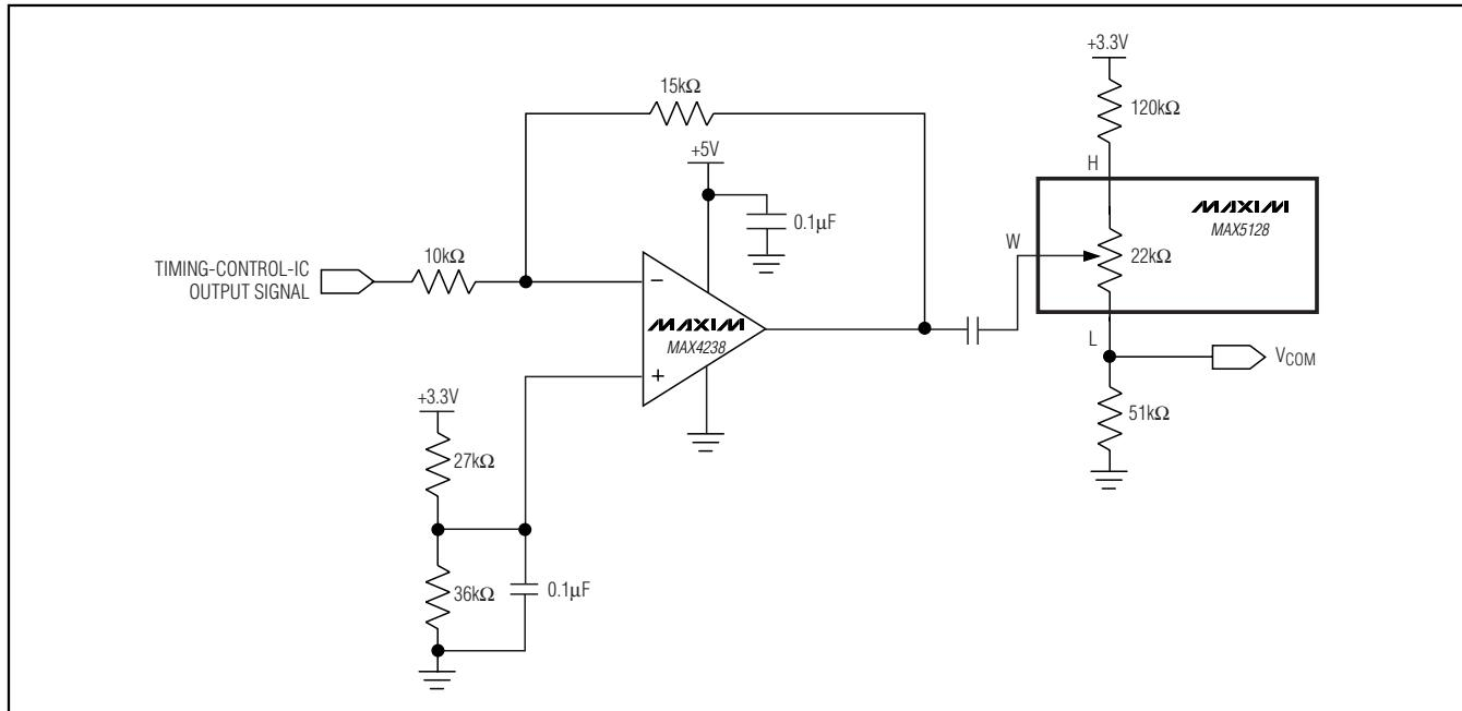
Figure 5. VCOM Generator Circuit for LCD Panels
