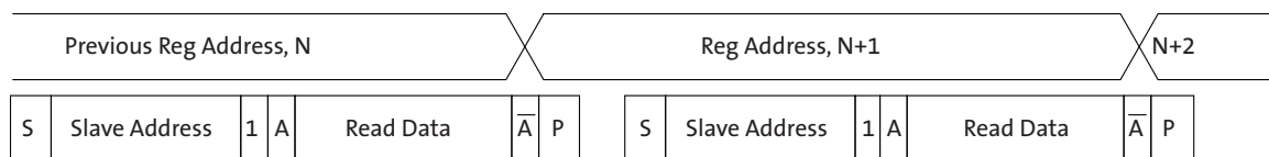
Figure 17: Single READ From Current Location
