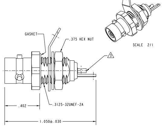
4. SUBMINIATURE TRIAXIAL SOLDER POT BULKHEAD MOUNT 3-LUG RECEPTACLE (TPS STYLE)
