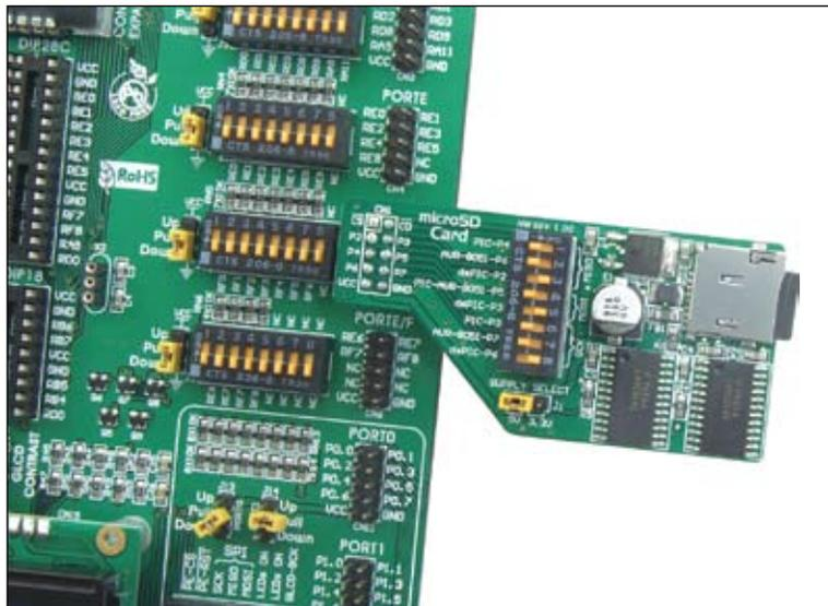
Figure 4: microSD Card connected to a development system
