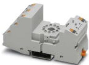
RIF-3... relay base, for octal relay with 3 PDTs, push-in connection, plug-in option for input/suppressor modules, for mounting on NS 35/7,5
