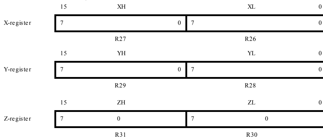
Figure 5-3. The X-, Y-, and Z-registers
