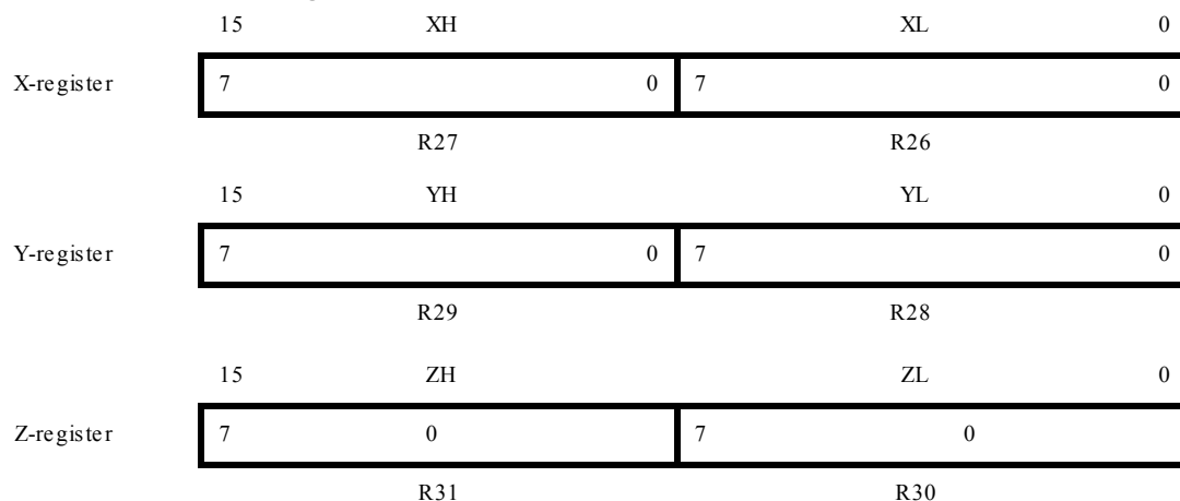
Figure 5-3. The X-, Y-, and Z-registers
