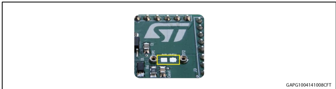
Figure 5: Pads for soldering SMD resistor
