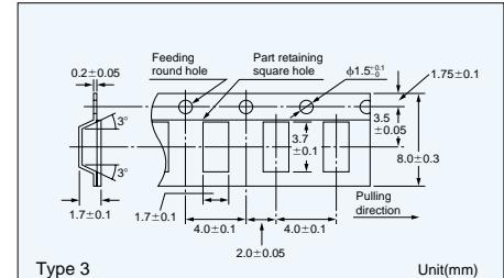
\*In principal elements are set with cathode side on the round hole side.
