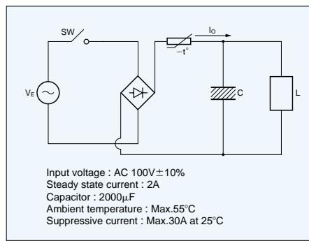
Accordingly, suitable thermistors are 6D-22, 5D-18 and 8D-18, and if we consider in the points of small time constant which means a small size and large effect for suppressive current which means large rated zero-power resistance, 8D-18 is the most suitable one.
