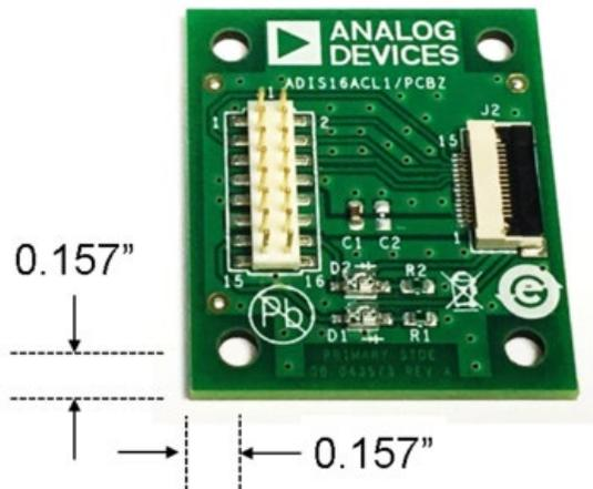
The basic diameter for the mounting holes (4x) is 0.130"
