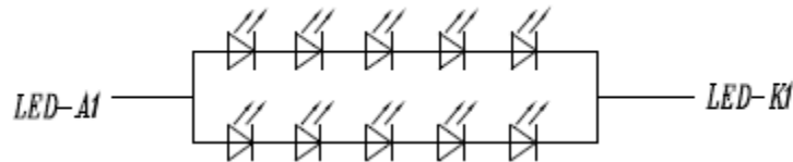
Figure: LED connection of backlight
