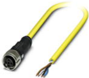
Sensor/Actuator cable, 4-position, PVC, Yellow RAL 1021, Free cable end, on Socket straight M12-SPEEDCON, A-coded, Cable length: 10 m
