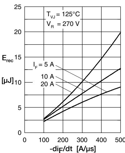
Fig. 7 Typ. recovery energy  $E_{rec}$  versus  $-di_F/dt$
