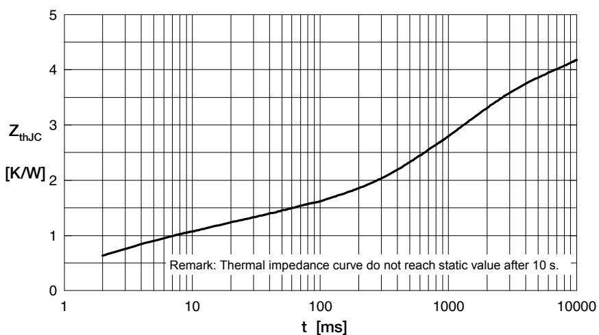
Fig. 8 Transient thermal resistance junction to case
