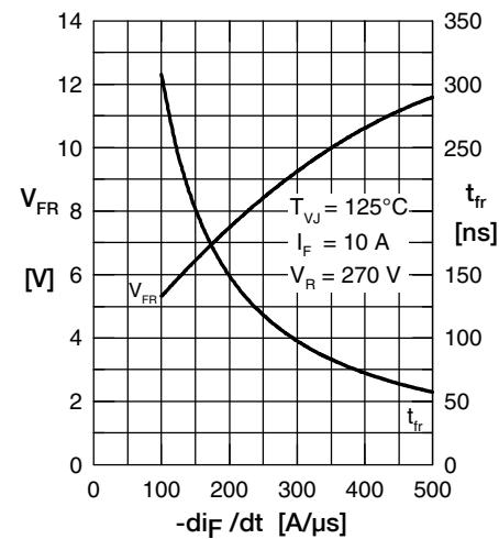
Fig. 6 Typ. forward recovery voltage  $V_{FR}$  and  $t_{fr}$  versus  $-di_F/dt$
