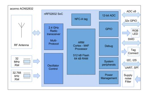
Solely the addition of a suitable DC power source is necessary for BLE and/or ANT connectivity. As a result of its Tag-Connect capabilities, the ease of application is increased further. Sensor applications require further addition of appropriate sensors. The NFC tag antenna can be connected externally.
