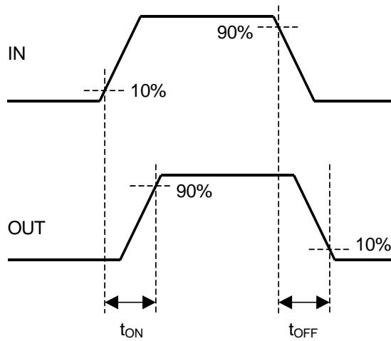
FLT Delay Time ( $V_{IN}=0$  to  $5V$ ,  $V_{DD}=V_{DS}=13V$ , FLT=Pull-up, OUT-GND shorting)
