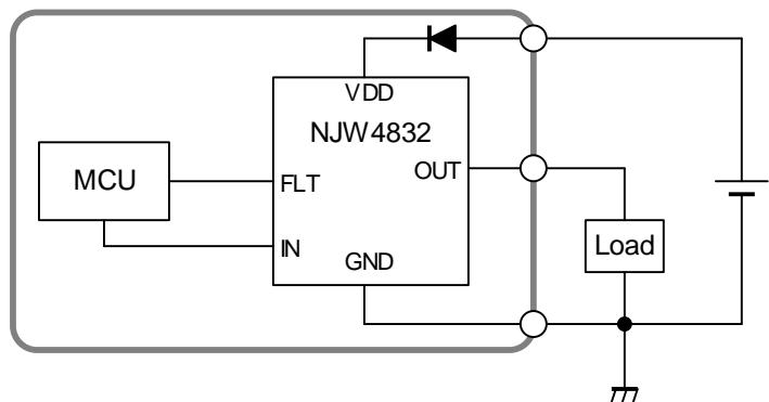
You should insert a pull-up resistor when you connect the FLT pin with other power supplies etc.
