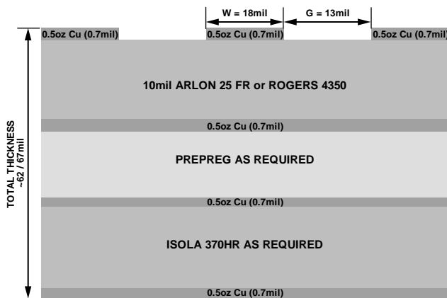
Figure 94. Evaluation Board Cross Sectional View
