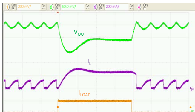
Figure 23. Load Transient 50mA to 250mA, V_{IN}=3V , t_{RISE}=t_{FALL}=100ns , 5μs/div.
