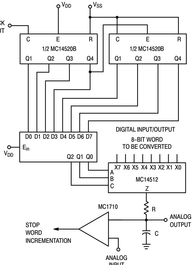
**Figure 6. Digital to Analog and Analog to Digital Converter**
