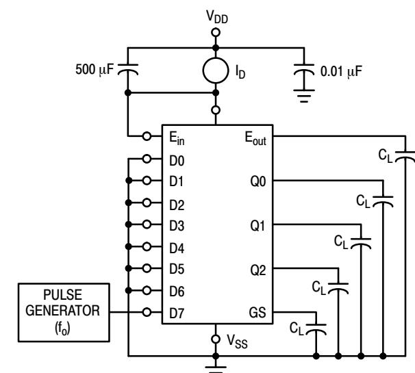
Figure 2. Typical Power Dissipation Test Circuit
