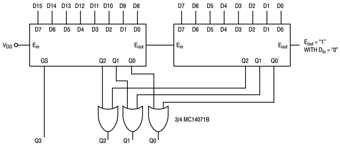
**Figure 5. Two MC14532B's Cascaded for 4-Bit Output**
