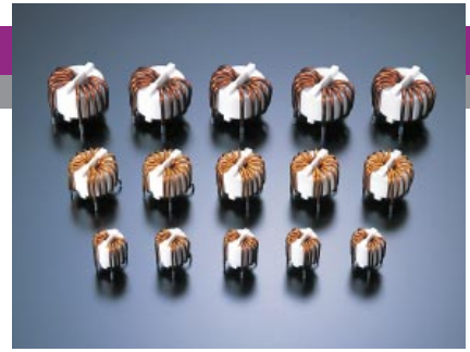
Item Specification Rated voltage AC250V or DC250V Insulation voltage rating AC1.5kV for 1min. or AC1.8kV for 3 sec. (line-line) Insulation resistance Over 100MΩ after applying DC500V for 1min. (line-line) Insulation grade Class E (120℃) Temperature rise *45℃ Operating temperature range -40℃ – +120℃ (including temperature rise of core)
