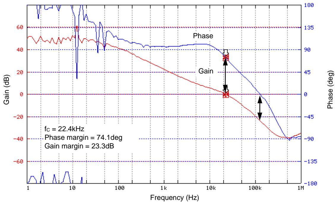
Figure 13. Loop Response  $V_{IN} = 12V$ ,  $V_O = 5.0V$ ,  $I_O = 2.5A$
