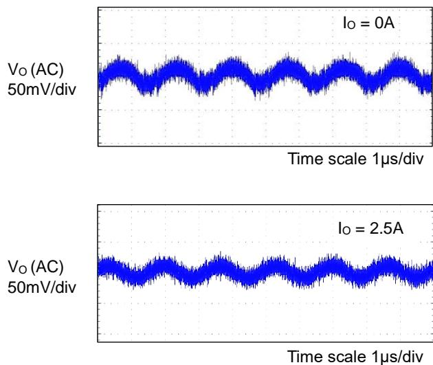
Figure 17. Output Voltage Ripple Wave
