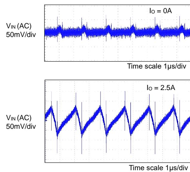
Figure 16. Input Voltage Ripple Wave
