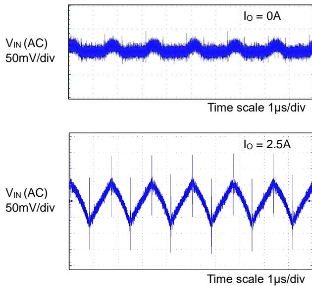
Figure 15. Input Voltage Ripple Wave
