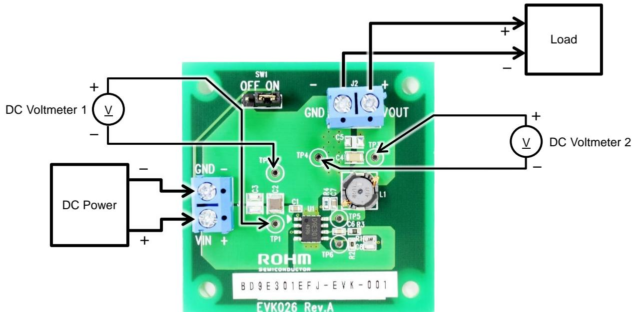
Figure 1. Connection Diagram
