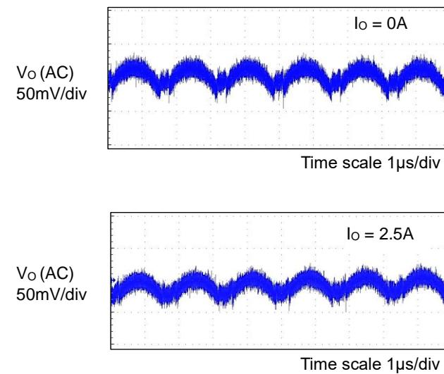
Figure 18. Output Voltage Ripple Wave
