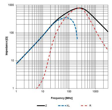
Test Equipment: E4991A or equivalent
