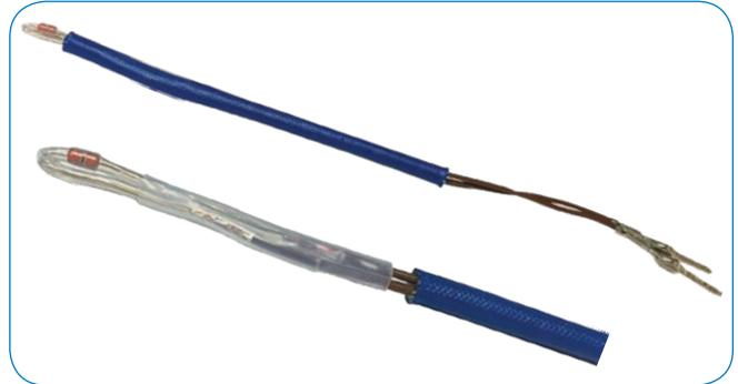
The A-1737 Motor Coil Temperature Sensor provides critical temperature feedback of an electric motor's operating condition. Used by either interlacing into the stator coil, or tied to the neutral bus bar on the motor circuit, it provides a temperature feedback to indicate motor load or stall conditions.
