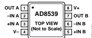
Figure 4. 8-Lead MSOP (RM-8)
