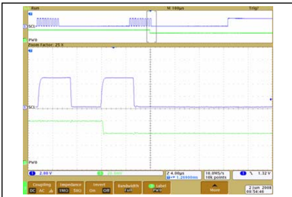
FIGURE 2-15: 5\text{ k}\Omega – Low-Voltage Decrement Wiper Settling Time ( V_{DD} = 2.7\text{V} ) ( 1\ \mu\text{s}/\text{Div} ).
