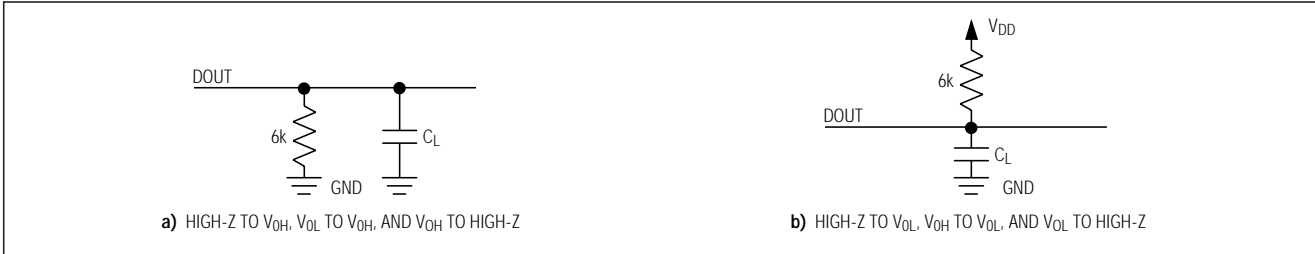
Figure 1. Load Circuits for Enable and Disable Time
