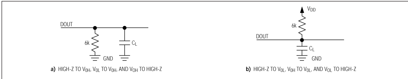
Figure 1. Load Circuits for Enable and Disable Time
