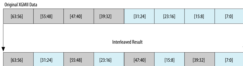
Figure 7-5: Interleaved SDR XGMII Data Mapping
