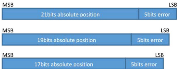
Figure 9: AR18 SSI 3-Wire Format Output
