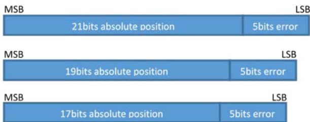
Figure 9: AR18 SSI 3-Wire Format Output
