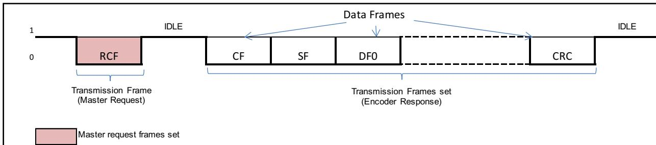
**Start of transmission frames set:** Upon detected the first logic of Low state 0 on the transmission line after idling state, and if the following 3 bit conforms to command identifier, the encoder will acknowledge as a valid Request Command Frame (RCF), indicating the start of transmission frame set; else, it will continue to search for next available logic of low state 0.
