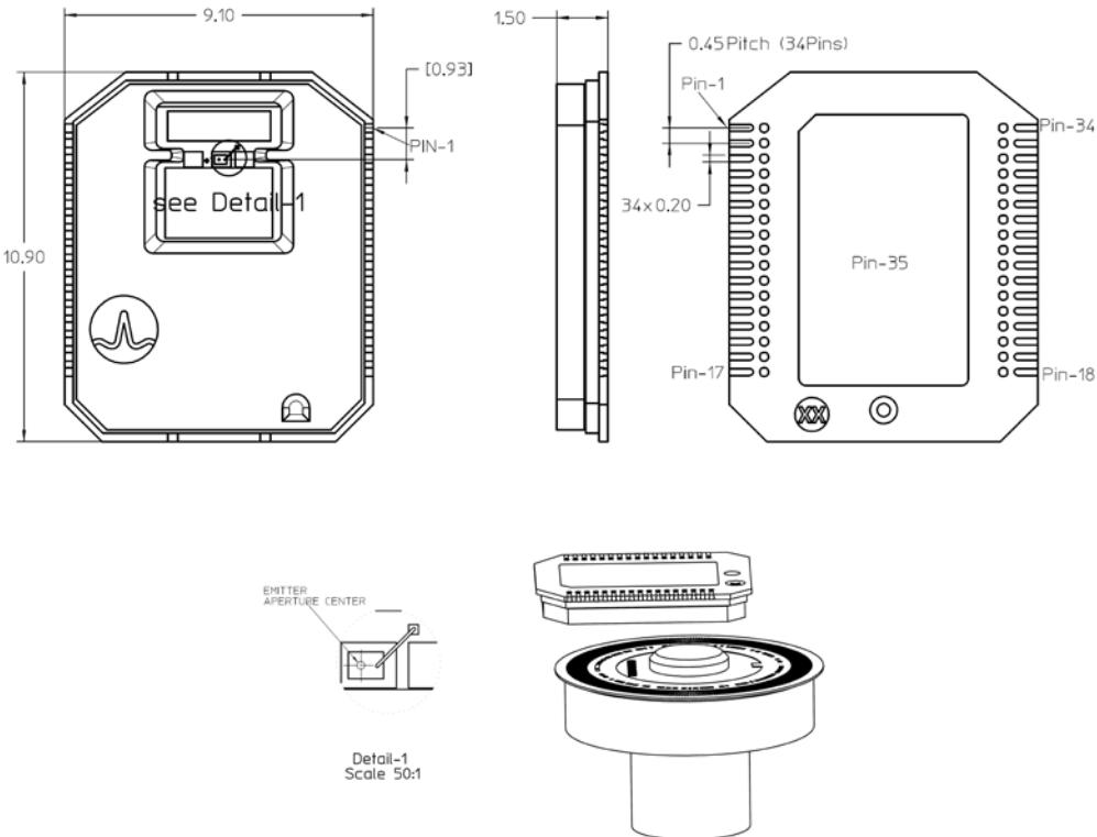
Note: All dimensions given in mm. Tolerances of form and position according to JEDEC MO-220.
