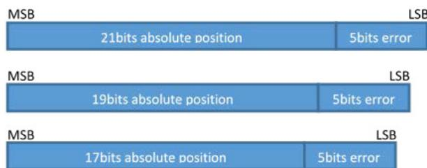
**Figure 10: AR35 SSI 3-Wire Format Output**
