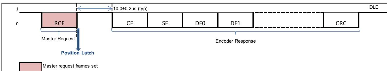
Upon the master issue a RCF frame request, after  $10.0 \mu s$  (typ.), the encoder will respond with encoder data frames set with the following content:
