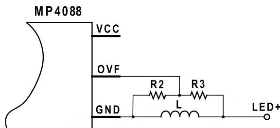
**Figure 7: Feedback Resistor Connection**
