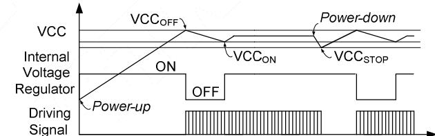
Figure 3: VCC Under-Voltage Lockout (UVLO)
