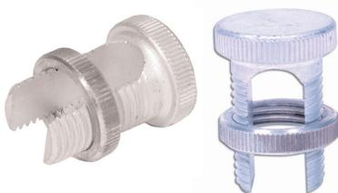
The slotted screw with knurled nut provides effective shield bonding of large aircore and filled service wires up to 1/2” shield O.D. (11, 16 and 25 pairs) to a ground wire or ground stud. Can also be used to bond the two pieces of butt spliced service drop within a buried service drop closure.
