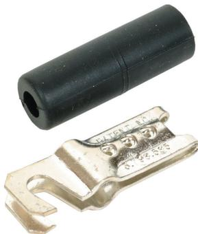
The one-piece clip, bonds or grounds the shield of a service wire or small cable up to 1/4” O.D. or 3/8” O.D. at station protectors, pedestals and similar terminations. Low resistance path to ground prevents stray electromagnetic interference from inducing noise or cross talk on cable pairs and provides a ground circuit path from the shield to the ground protector.
